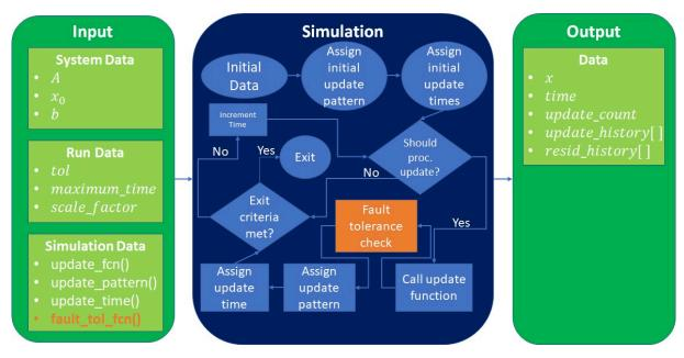
**Figure 10.** Block diagram of the simulation framework with added support for fault tolerance mechanisms.
