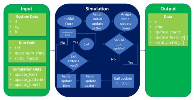
Figure 2. Block diagram of the simulation framework.
