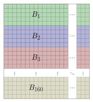
Figure 2. Block assignment used in the  $800 \times 800$  grid of the example problem. The blocks consist of all components in a five-row section of the grid. This incorporates 4000 of the 640,000 grid points into each block resulting in  $\hat{n} = 160$  blocks.
