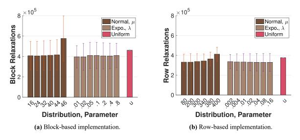
**Figure 15.** The average number of (a) block and (b) row relaxations required to converge for different probability distributions and parameters for the two implementations. The vertical lines in each bar show the standard deviation of the number of row relaxations among all rows.
