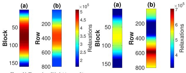
**Figure 16.** The number of block (a) or row (b) relaxations required to converge with good normal distribution parameters.
