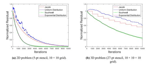
**Figure 1.** Residual  $(r / r_0)$  progression for the first 10,000 iterations of four stationary methods solving the 2D (a) and 3D (b) Laplacian.
